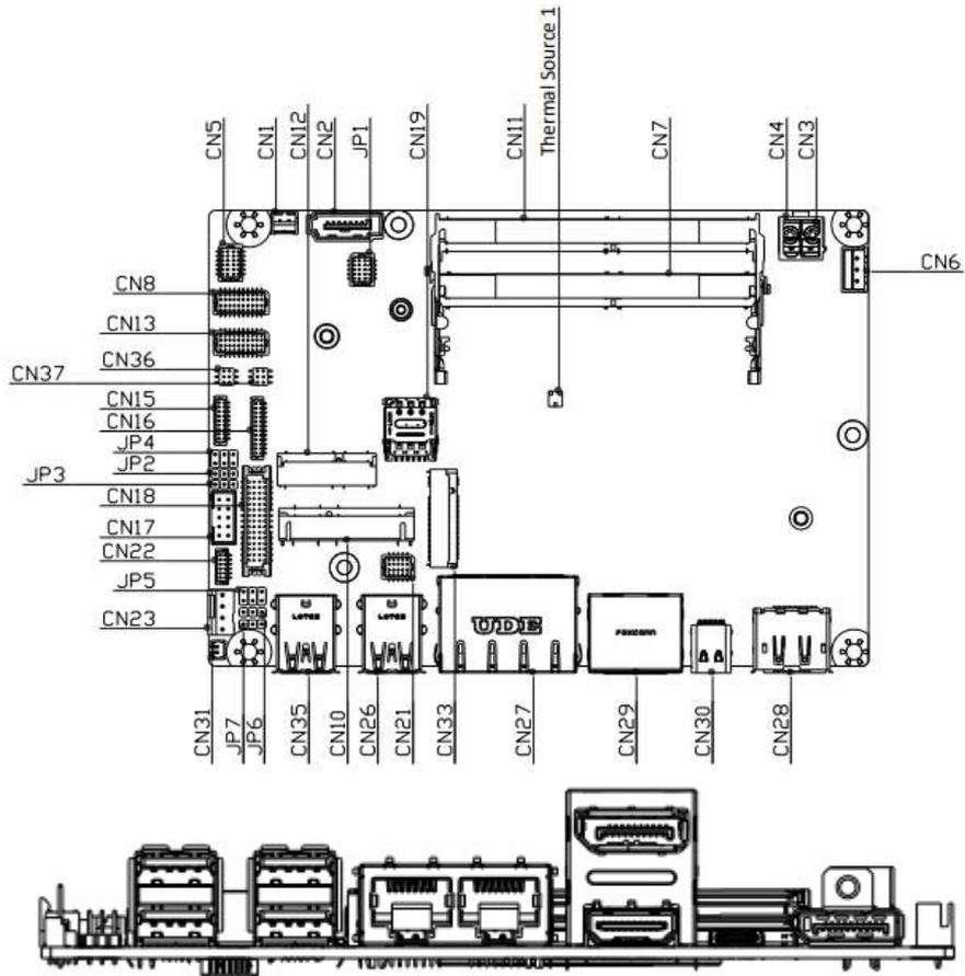
Figure 2.2: Jumpers and Connectors Location- Board Top
